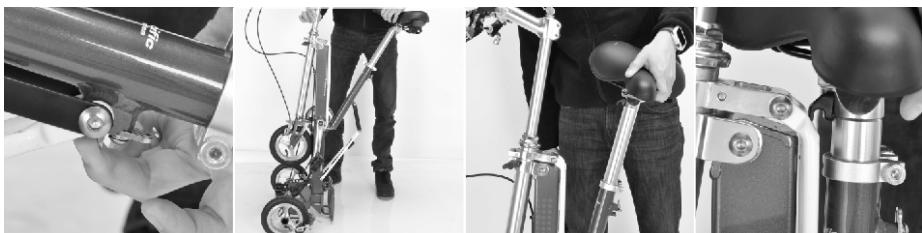
Step 3. Open the stem QR lever, turn the handle  $180^{\circ}$  then lower the stem and close the QR. Open the handlebar clamp QR, pull out the side bars to reduce the width of handlebar.
