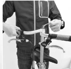
Step 2. Open the QR lever on the seat tube and raise the seat post to the appropriate height. Swing the seat tube backwards. Lock the seat stays to the seat tube linkage fixing latch.
