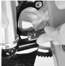
Step 2. Unlock the seat post from seat stay. Pull the seat toward the handlebar, open the seat clamp QR lever, lower the seat and turn it side ways, hook the seat to the head tube stay.
