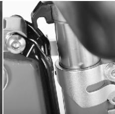
Step 3. Open the stem QR lever, lower the stem and turn the handlebar top of saddle. Close the QR.
