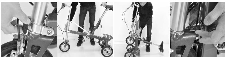
Step 2. Unlock the seat post from seat stay. Pull the seat toward the handlebar, open the seat clamp QR lever, lower the seat and turn it side ways, hook the seat to the head tube stay.
