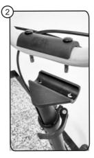
Place the handlebar set and stem top cap on the folding stem
