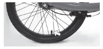
NOTE: Tire pressure may affect the riding performance. Lower pressure makes for a comfortable but slower ride, higher pressure makes for a faster but slightly bumpier ride. Use a tire gauge. Do not ride with the pressure too low.
