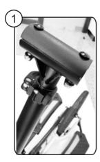
Unscrew the nut with the attached hexagon wrench and open the stem top cap
