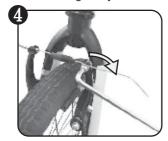
Tighten the screw clockwise
