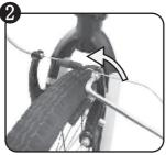
Loosen the screw counterclockwise gentely
