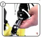
Press the quick release lever inwards firmly.
