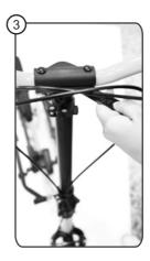
Tighten the screws with the attached wrench.
